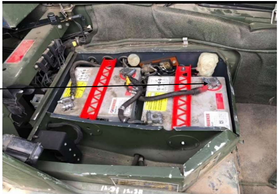
Picture of CLB-453 HMMWV with 3D printed battery bracket.
