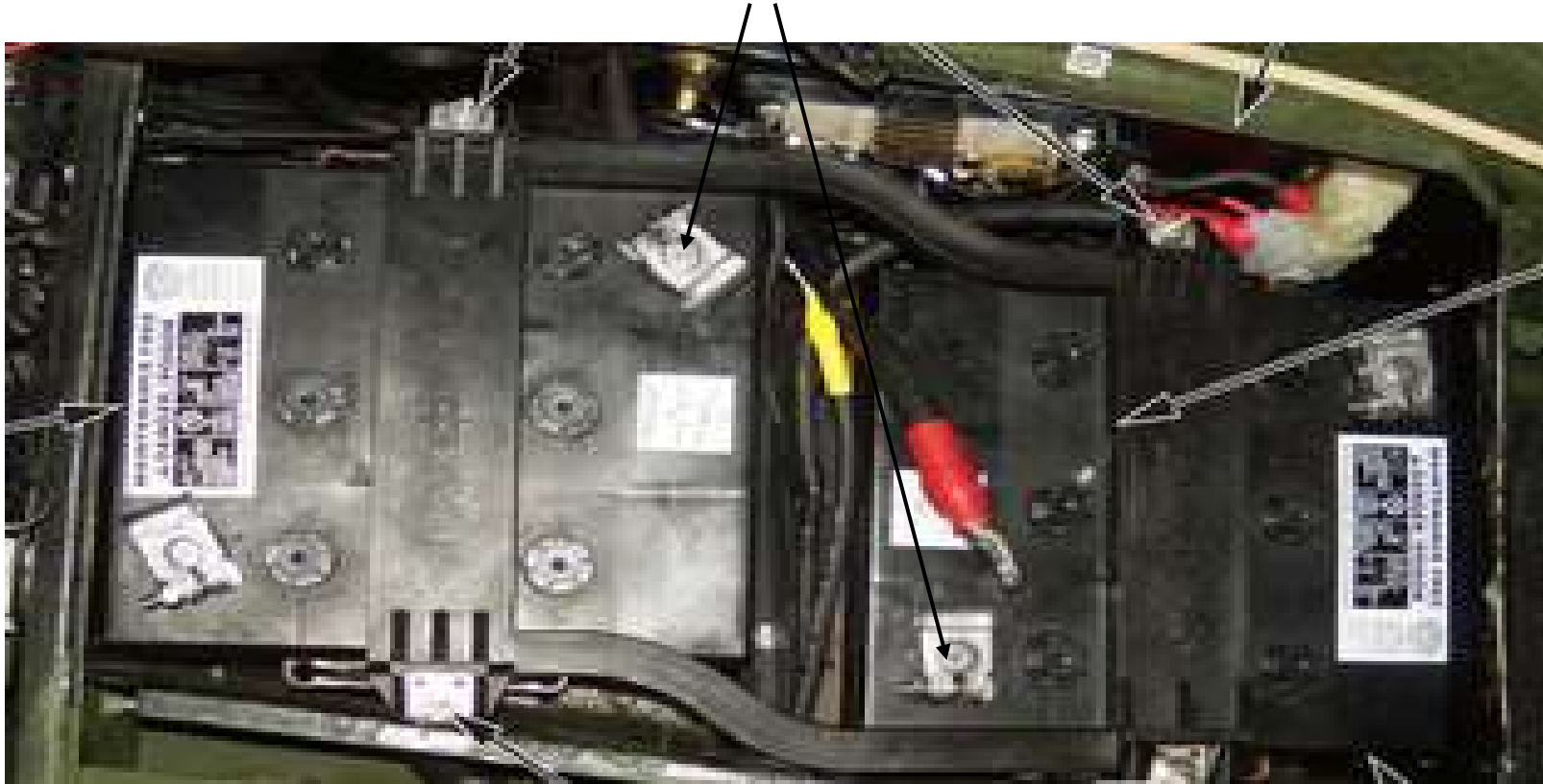
IETM Picture of properly installed batteries.
